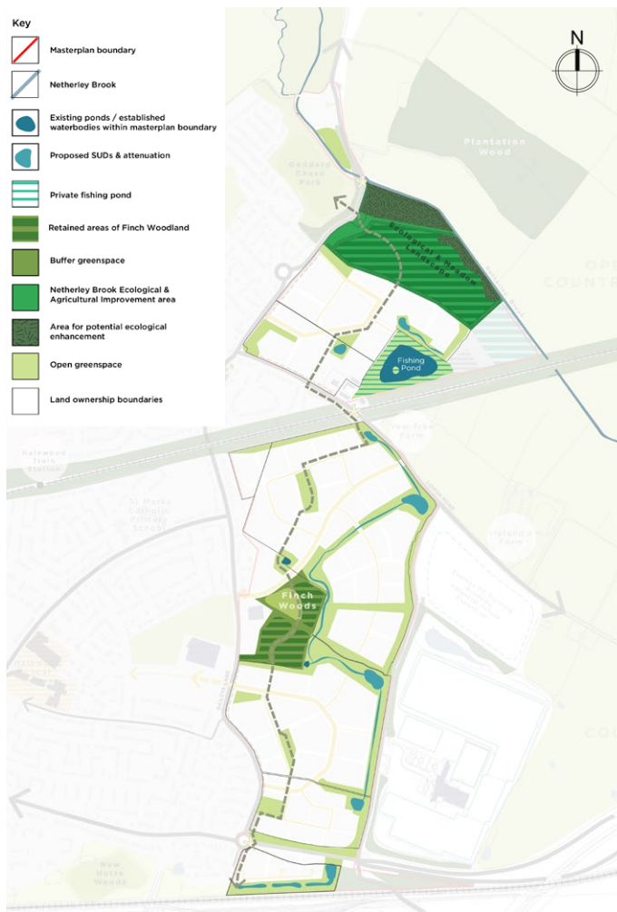
Figure 7.6 Surface water drainage management
